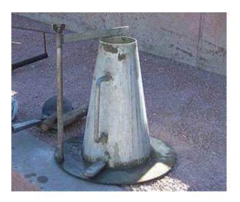
Figure 2 SLUMP CONE
